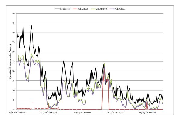
Figure 1: Time series chart of hourly mean sensor and reference PM<sub>2.5</sub> concentrations over the test period prior to application of scaling factors.
