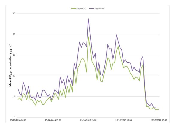
Figure 4: Time series chart of one-minute sensor PM<sub>2.5</sub> concentrations over the one-hour mobile monitoring campaign.
