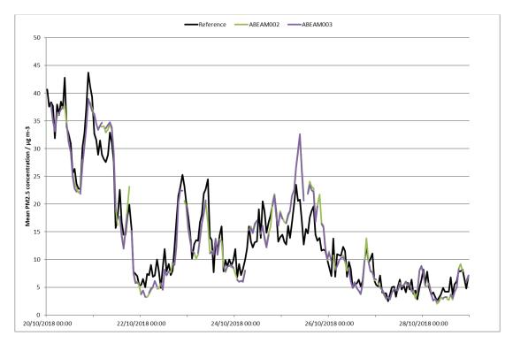
Figure 2: Time series chart of hourly mean sensor and reference PM<sub>2.5</sub> concentrations over the test period following application of scaling factors. ABEAM001 is excluded due to this sensor being defective.
